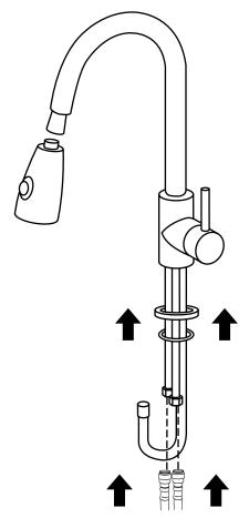
\*Remember to install the 'O' ring o washer between the mixer body & sanitary ware\*
